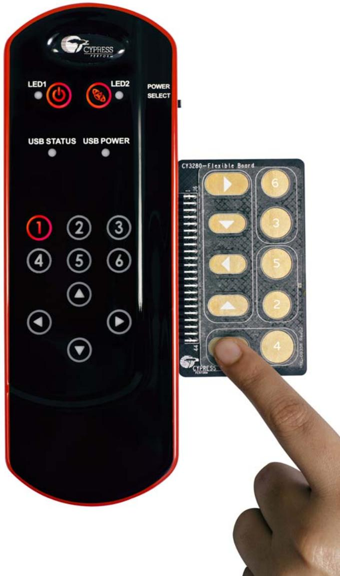
SmartSense Auto-Tuning algorithm can also be tested on the Simple Button Module (BSM) board. The BSM board can be connected to the kit and tested for SmartSense Auto-Tuning in the same way as the Flex-PCB. BSM board is not provided as part of this kit. To purchase or know more about BSM board, refer to the [Cypress website](#). The Flex-PCB needs to be disconnected from the kit to test the features mentioned in the subsequent sections.
