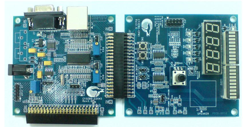
2. Connect your PC to the CY3280-22x45 Universal CapSense Controller board's ISSP connector (J3) using a PSoC MiniProg and an USB cable.
