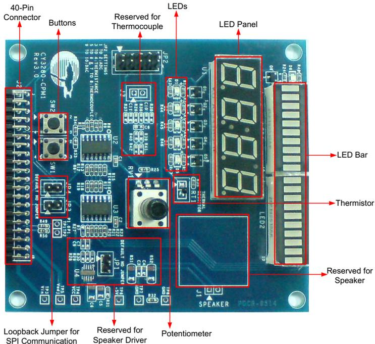
The module board consists of an LED panel, a potentiometer, an LED bar, six LEDs, a thermistor, and two buttons. These are interfaced to the CapSense Controller board via a 40-pin receptacle connector (J2). The board also consists of two loop-back connection jumpers (JP3 and JP4) to demonstrate the variable length SPI master-slave communication.
