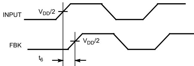
Figure 8. Device-Device Skew
