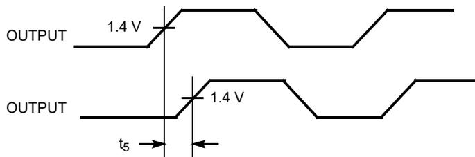
Figure 7. Input-Output Skew
