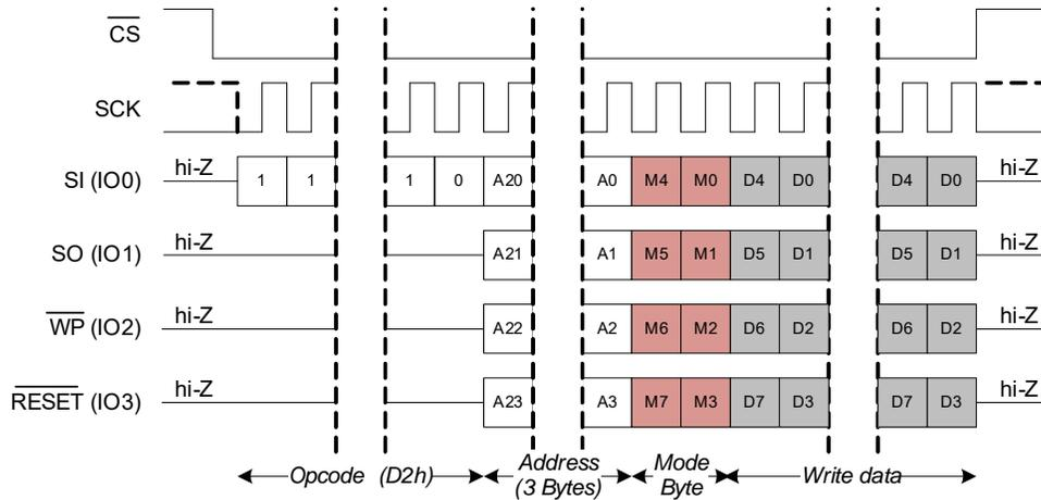
**DDR Quad I/O Write (DDRQIOW, D1h)**
