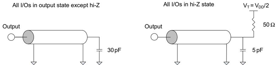
**Figure 114. AC Timing Input Voltage Reference Levels**
