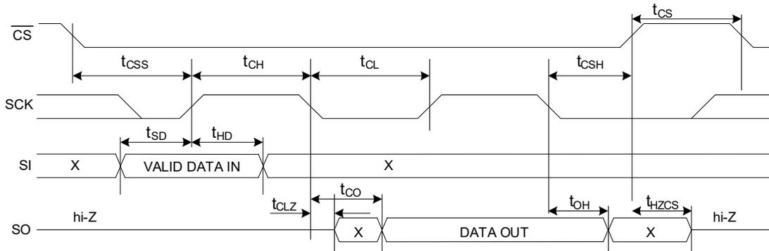
Figure 116. SPI Switching Timing - Multiple I/O, SDR
