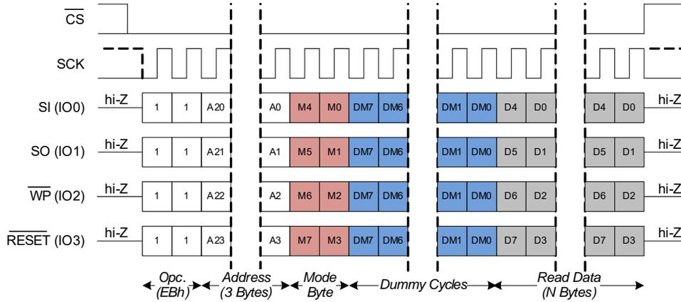
**Quad I/O Read (QIOR, EBh) – In Extended SPI Mode**
