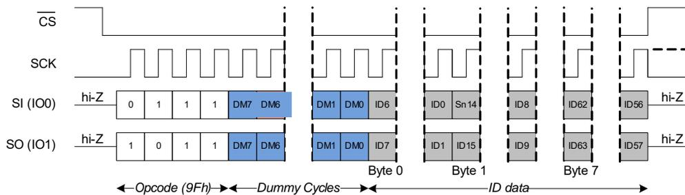
**Figure 90. Read Device ID (RDID) in QPI Mode**
