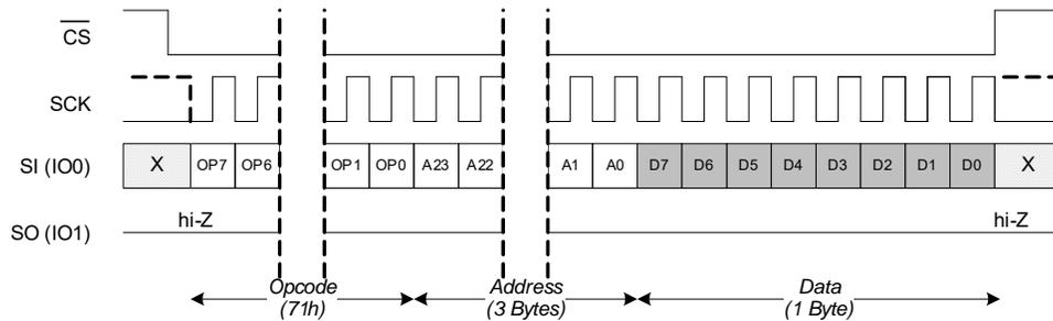
**Figure 35. Write Any Register (WRAR) in DPI Mode**
