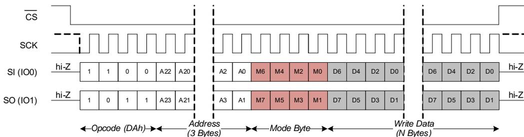
Figure 46. Fast Write (FAST\_WRITE) in QPI Mode
