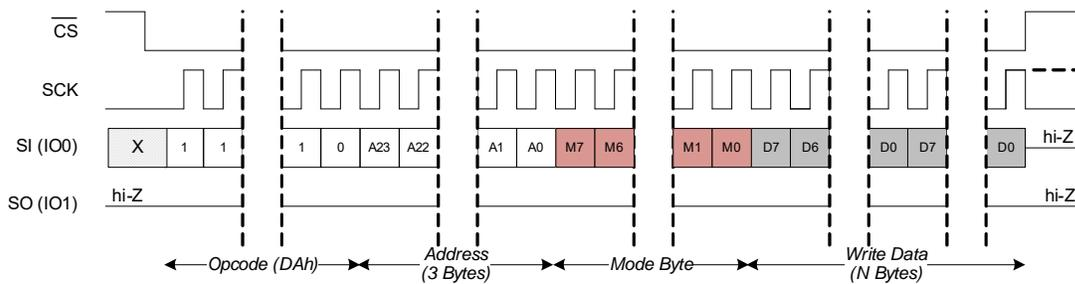
Figure 45. Fast Write (FAST\_WRITE) in DPI Mode
