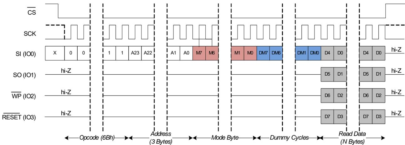
**Quad I/O Read (QIOR, EBh) – In Extended SPI Mode**
