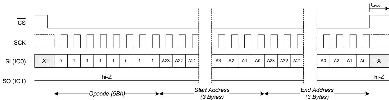
Figure 80. CRC Calculation (CRCC) in DPI Mode
