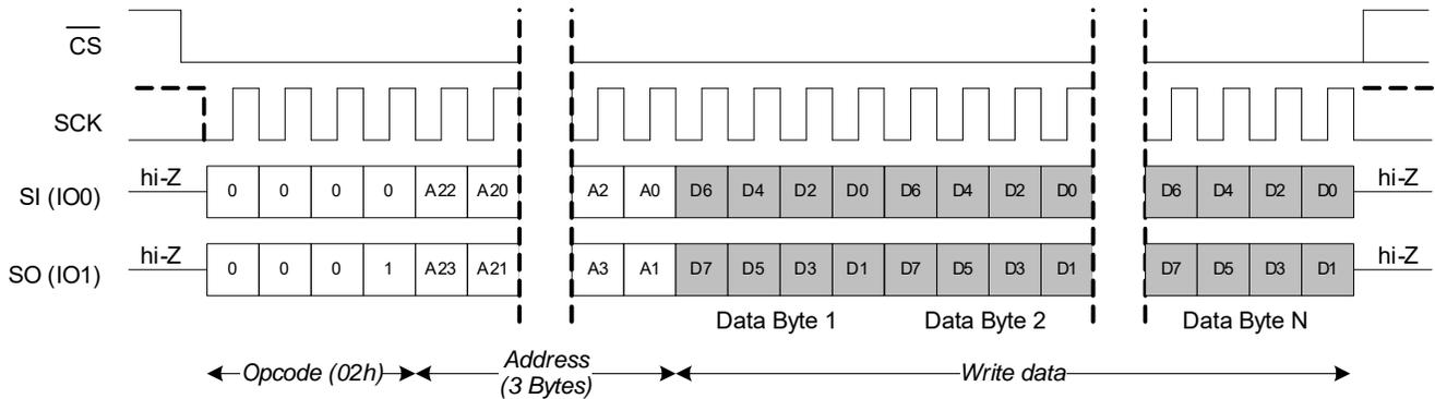
Figure 42. Memory Write (WRITE) in QPI Mode
