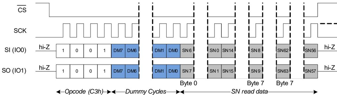
**Figure 99. Read Serial Number (RDSN) in QPI Mode**
