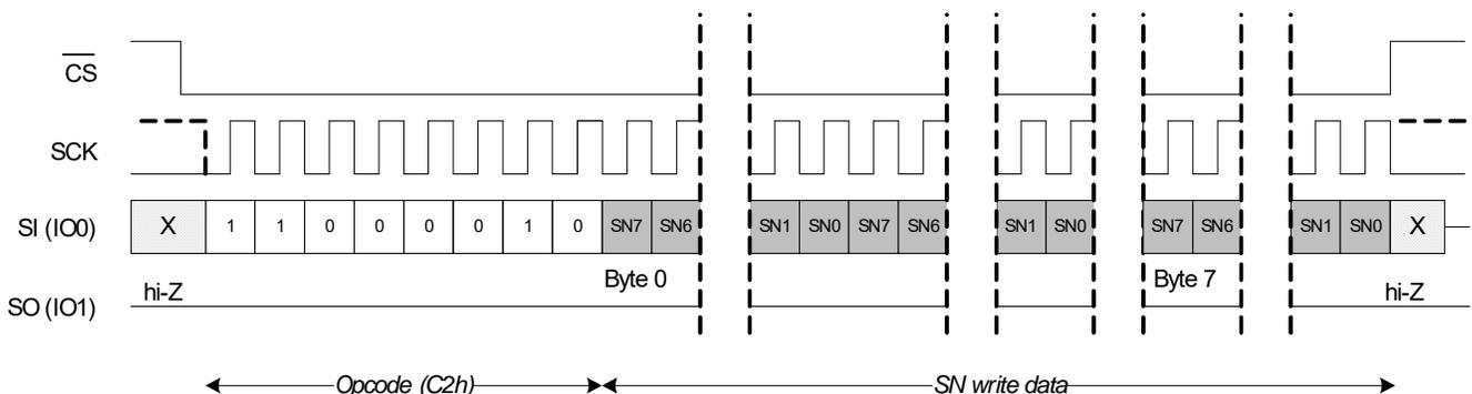
**Figure 95. Write Serial Number in DPI Mode (WREN not shown)**
