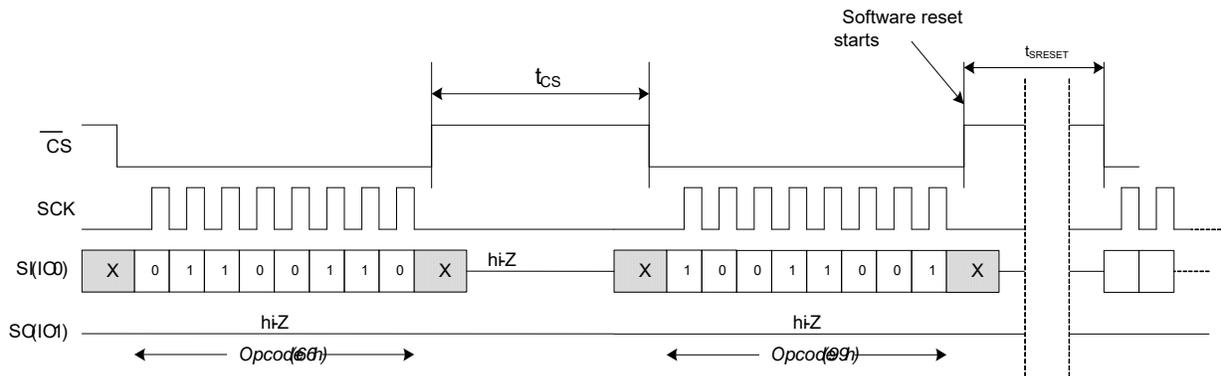
**Figure 108. Software Reset Timing in DPI Mode**
