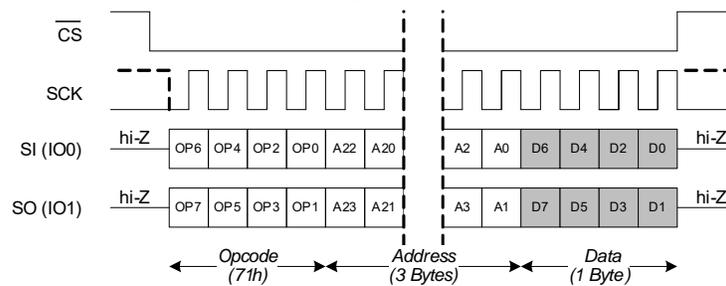
**Figure 36. Write Any Register (WRAR) in QPI Mode**
