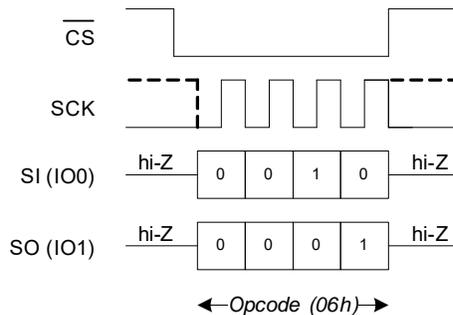
Figure 9. WREN Bus Configuration in QPI Mode
