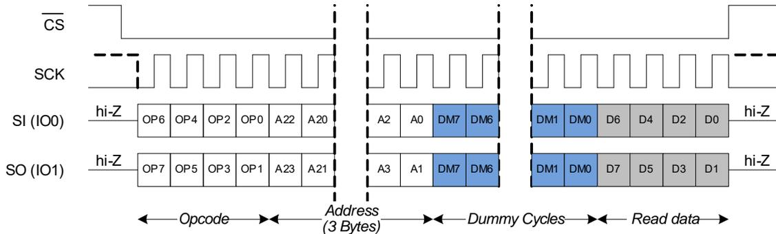
**Figure 39. Read Any Register (RDAR) in QPI Mode**
