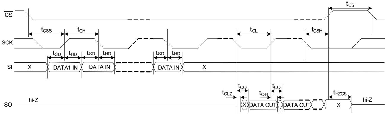
Figure 119. SPI Switching Timing - Multiple I/O, DDR <sup>[24]</sup>
