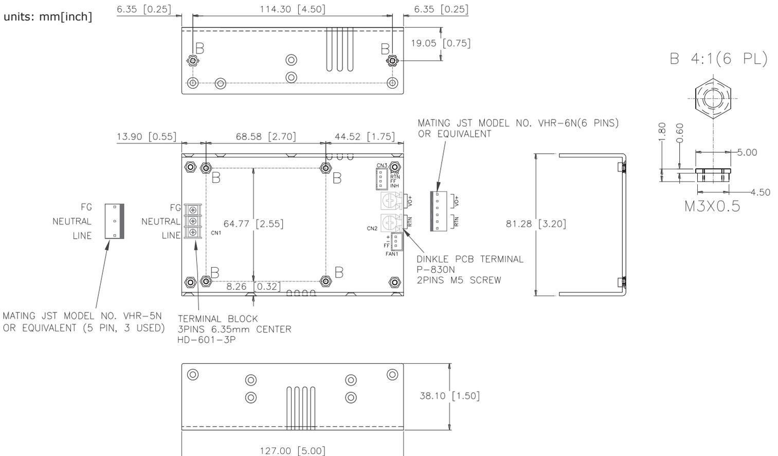
Note: 1. Mounting hole max screw depth is 4.0mm (M3x0.5 Inserts).
