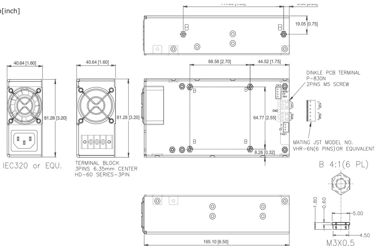
Note: 1. Mounting hole max screw depth is 4.0mm (M3x0.5 Inserts).
