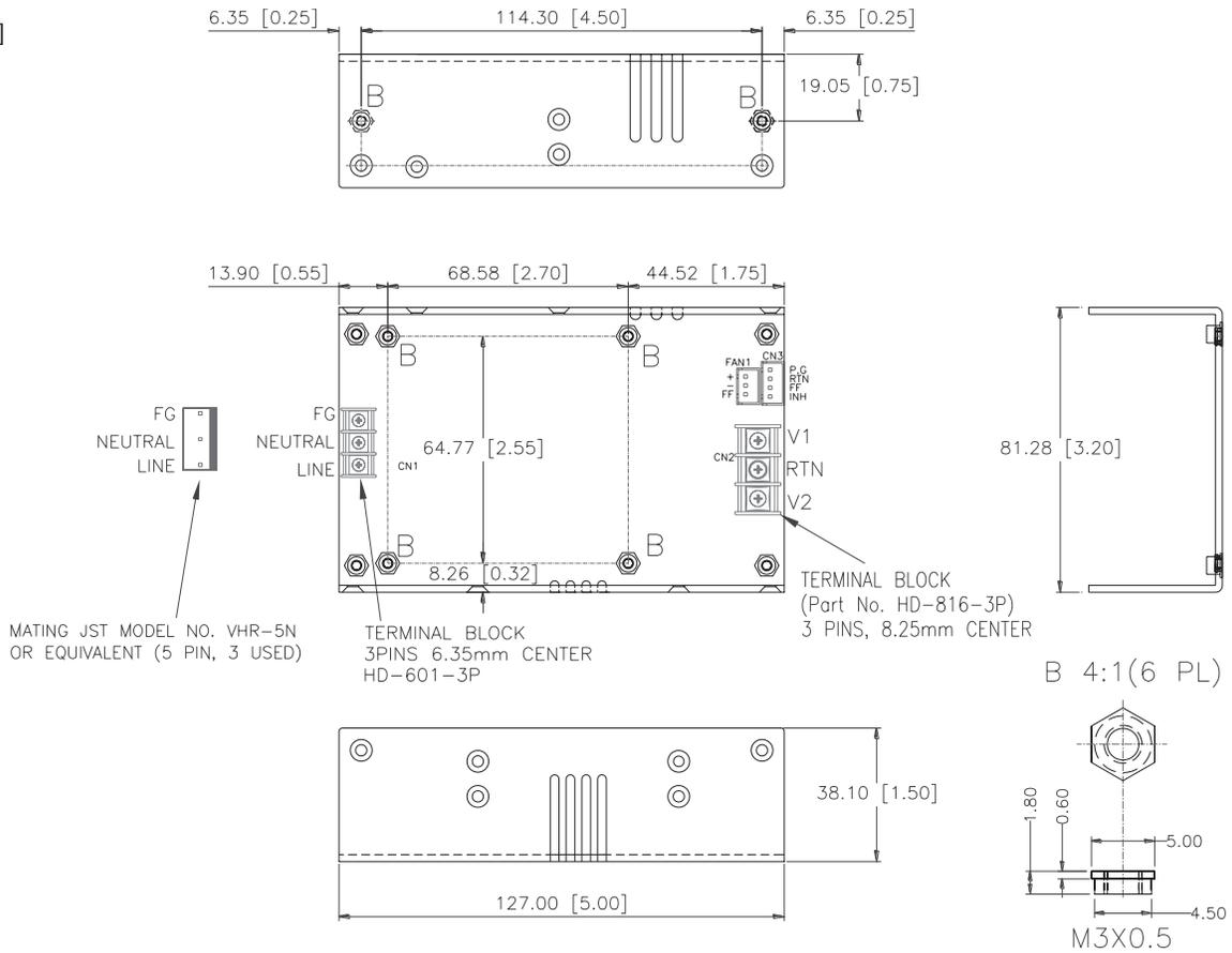
Note: 1. Mounting hole max screw depth is 4.0mm (M3x0.5 Inserts).
