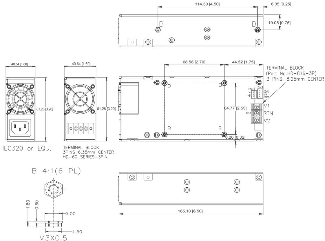
Note: 1. Mounting hole max screw depth is 4.0mm (M3x0.5 Inserts).
