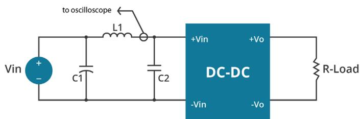
Figure 2 Measuring Output Ripple And Noise
