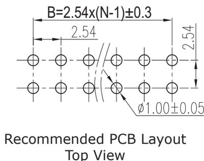
This series is constructed of single piece modules where L is the total length, P is the pitch, and N is the number of poles.
