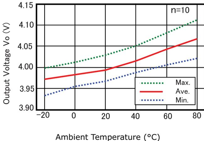
Offset Voltage vs. Ambient Temperature
