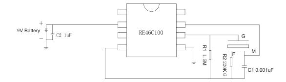
Notes: 1. The current consumption and the sound pressure level are measured by using the recommended driving circuit shown above.
