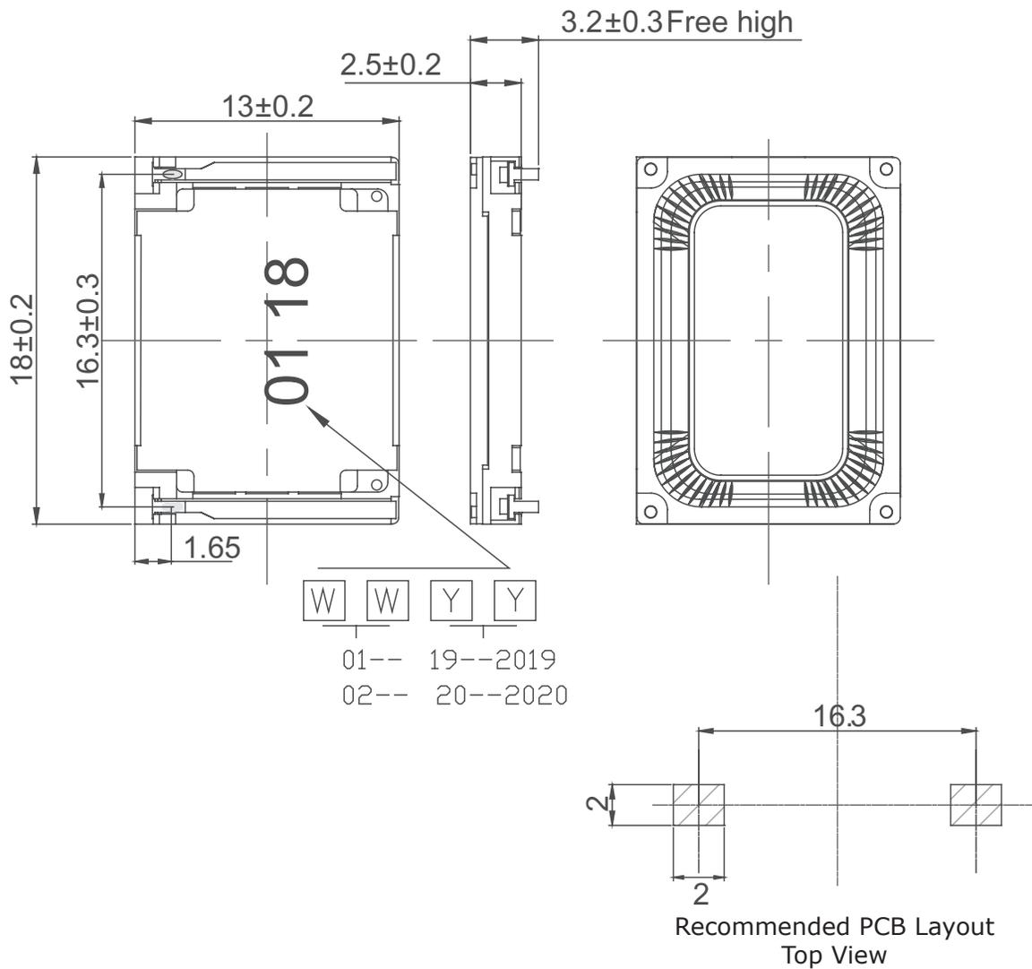
Note: 1. Maximum compression force between front frame and back frame & yoke is 5 N.
