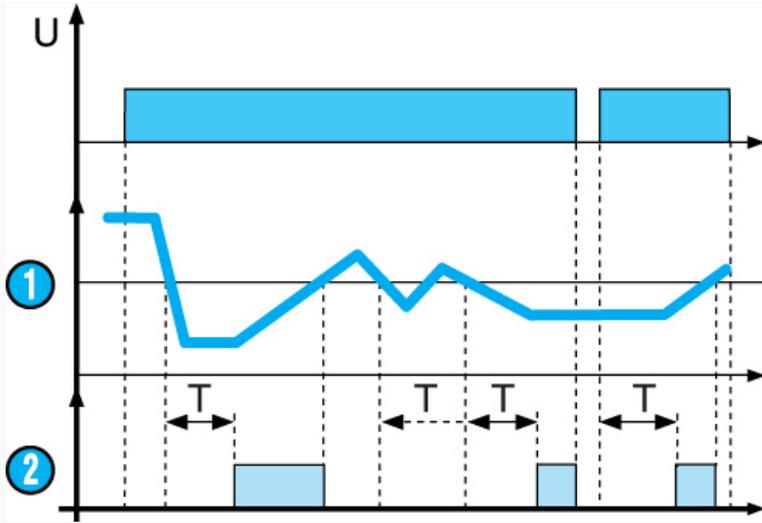
**Monitoring a level, filling function, activation time**
