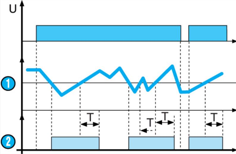
**Monitoring a level, filling function, deactivation time**
