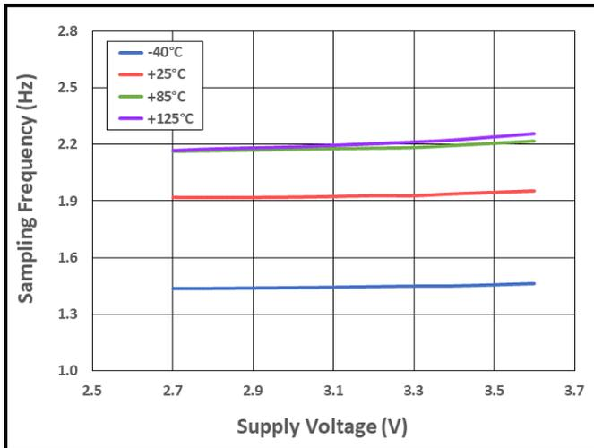
**Figure 7.** Sampling Frequency vs. Supply Voltage vs. Temperature
