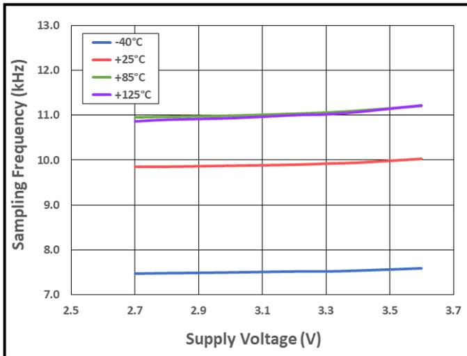
**Figure 39.** Sampling Frequency vs. Supply Voltage vs. Temperature
