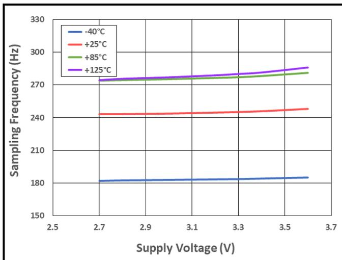
**Figure 21.** Sampling Frequency vs. Supply Voltage vs. Temperature
