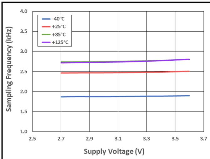
**Figure 32.** Sampling Frequency vs. Supply Voltage vs. Temperature
