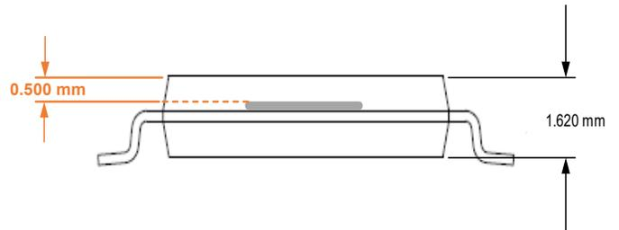
Figure 41. XtremeSense TMR Current Sensor Location in z Dimension for CT453 in SOIC-8 Package
