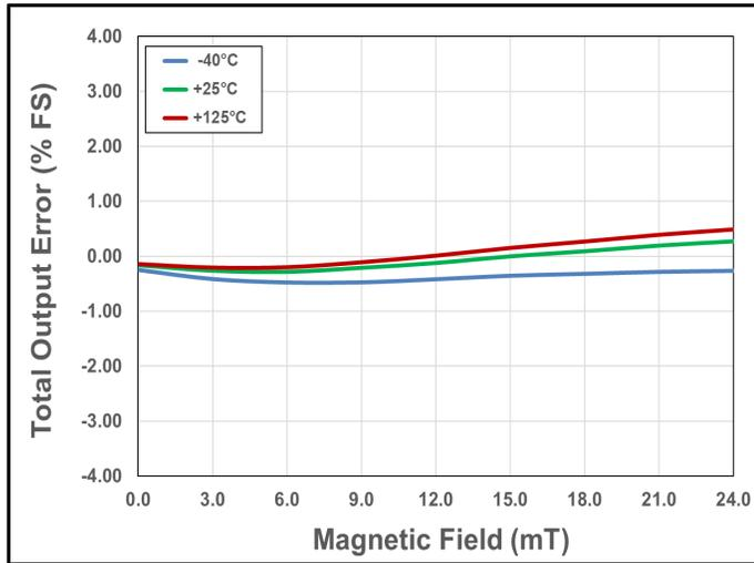
Figure 19. Total Output Error vs. Current vs. Temperature
