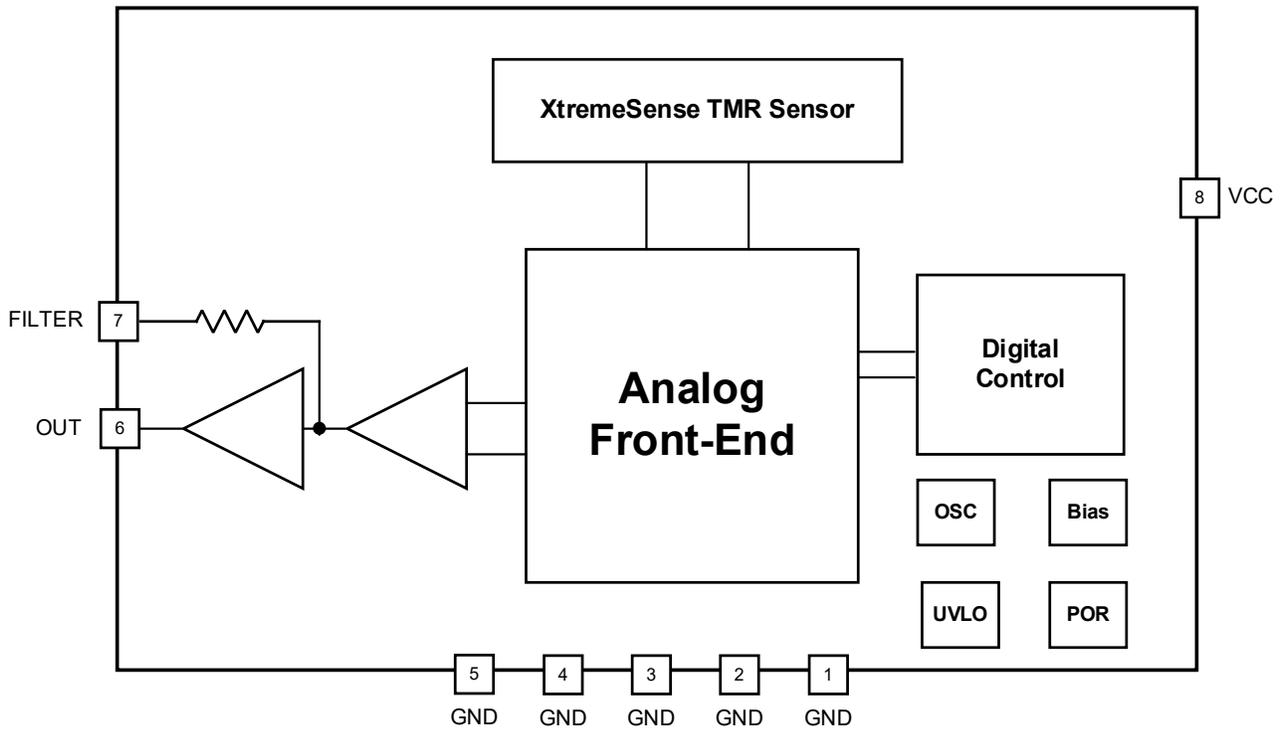
Figure 1. CT453 Functional Block Diagram for SOIC-8
