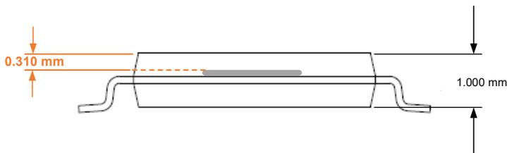
**Figure 43. XtremeSense TMR Current Sensor Location in z Dimension for CT453 in TSSOP-8 Package**
