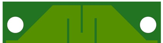
Figure 25. PCB Trace Design to Generate Differential Magnetic Field for CT453 to Measure
