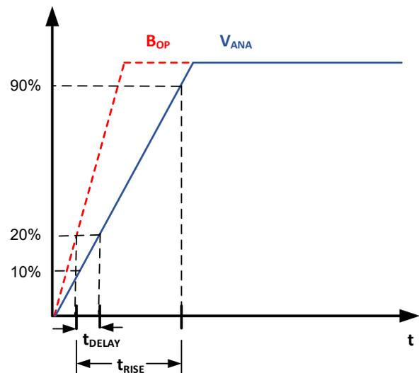
**Figure 30. CT453 Propagation Delay and Rise Time Curve**
