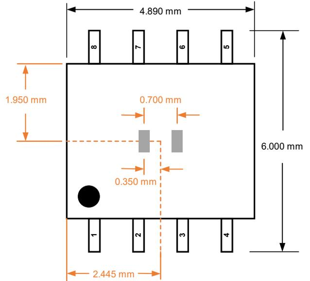
Figure 40. XtremeSense TMR Current Sensor Location in x-y Plane for CT453 in SOIC-8 Package
