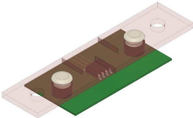
**Figure 27. CT453 for Contactless Current Sensing Using Busbar**
