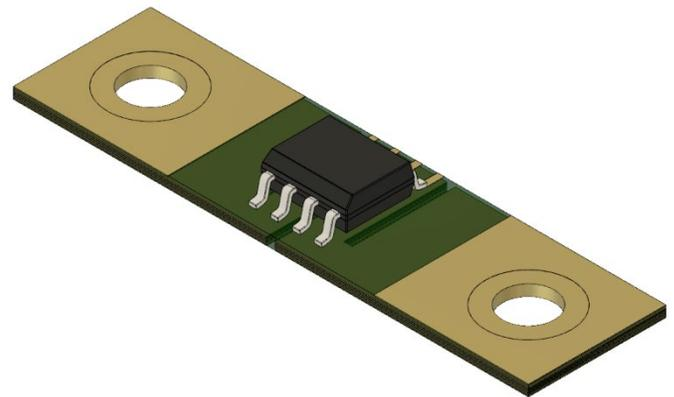
Figure 24. 3D View of CT453 and PCB Trace Design
