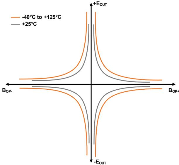
**Figure 28. Total Output Error ( $E_{OUT}$ ) vs. Field ( $B_{OP}$ )**
