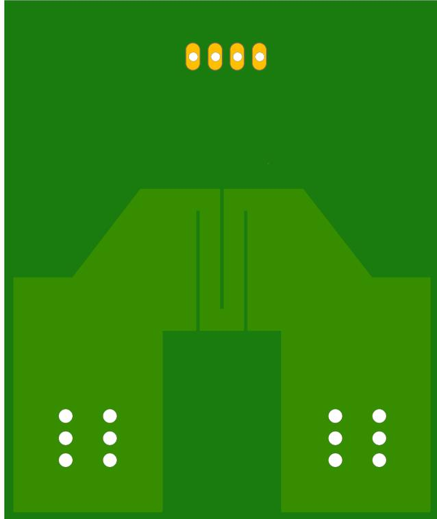
Figure 39. Recommended PCB Layout (Bottom Layer) for CT453
