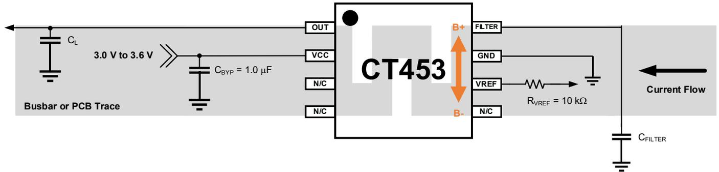
Figure 4. CT453 Application Diagram for TSSOP-8
