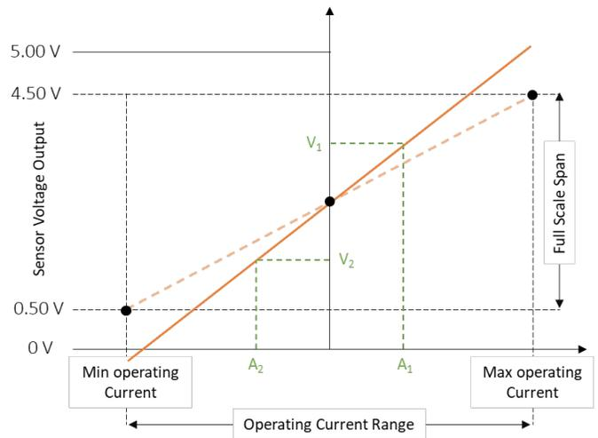
Figure 36. Gain Calibration
