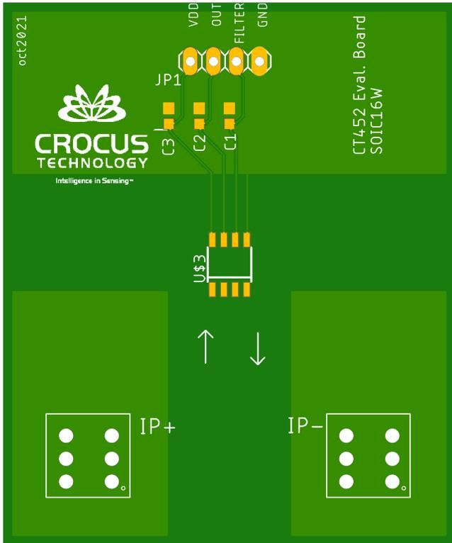
Figure 38. Recommended PCB Layout (Top Layer) for CT453
