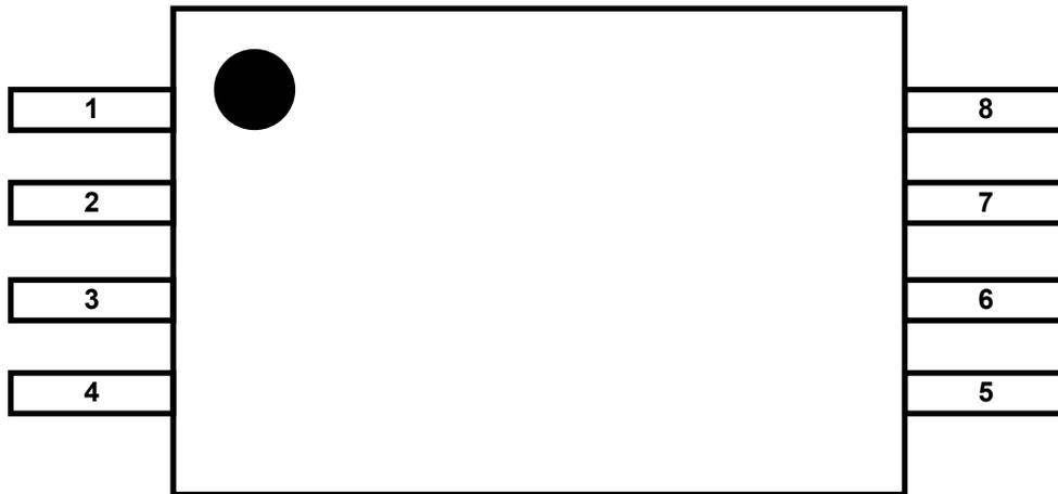
Figure 6. CT453 Pin-out Diagram for 8-lead TSSOP Package (Top-Down View)
