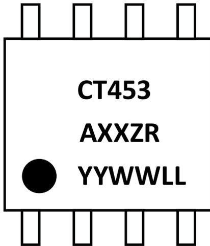
Figure 48. CT453 Device Marking for 8-lead SOIC Package
