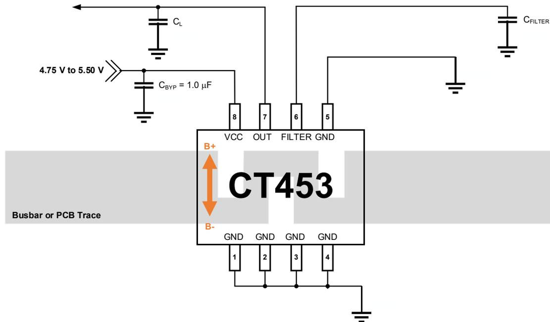
Figure 37. Application Diagram of CT453 Sensing Current of Busbar or PCB Trace Underneath It
