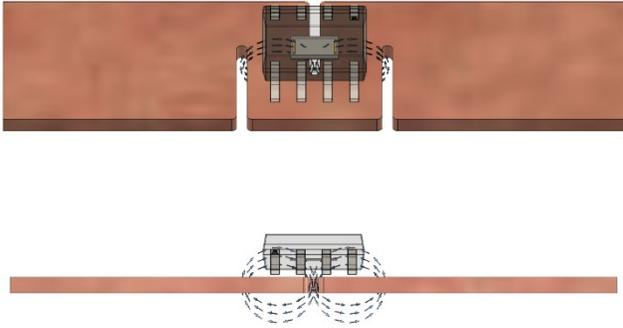
**Figure 26. Differential Magnetic Fields Generated Current Through the Busbar (or PCB Trace) and Measured by the CT453**
