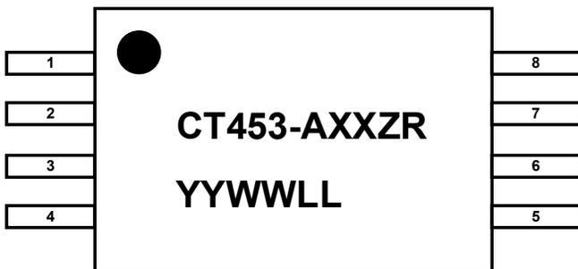
Figure 49. CT453 Device Marking for 8-lead TSSOP Package
