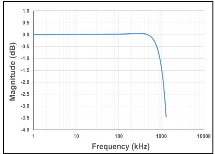
Figure 8. CT453 Bandwidth with  $C_{FILTER} = 1.0\ \text{pF}$
