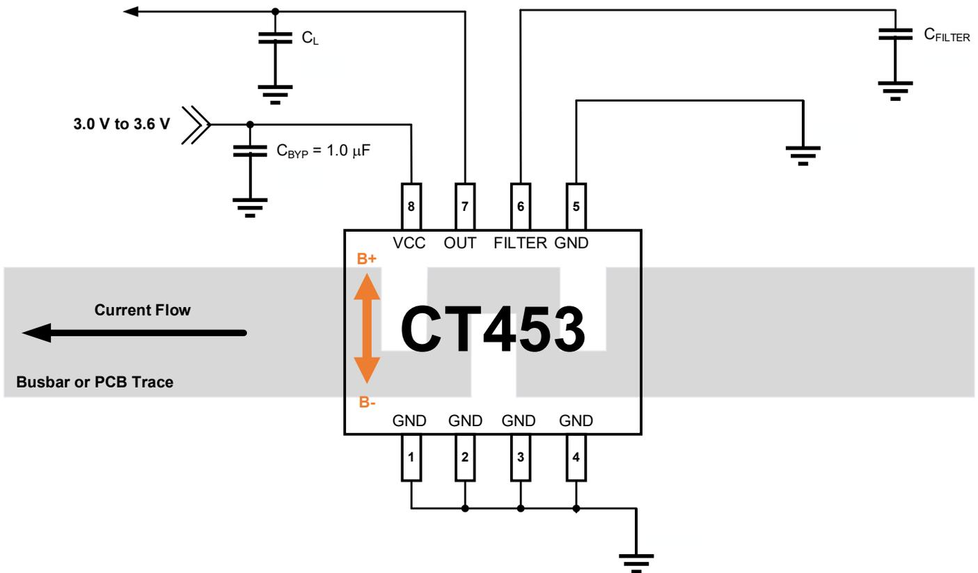
Figure 3. CT453 Application Diagram for SOIC-8
