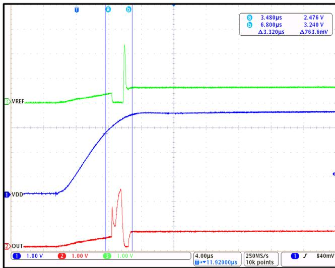
Figure 9. CT453 Startup Waveforms for  $V_{OQ} = 0.65\ \text{V}$  (Unipolar Field)
