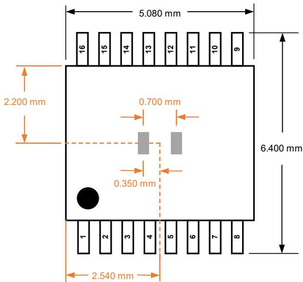
**Figure 42. XtremeSense TMR Current Sensor Location in x-y Plane for CT453 in TSSOP-8 Package**
