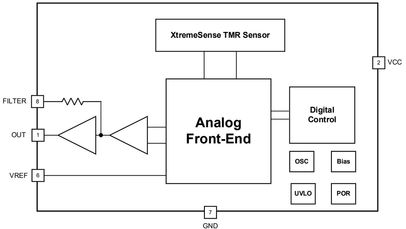
Figure 2. CT453 Functional Block Diagram for TSSOP-8
