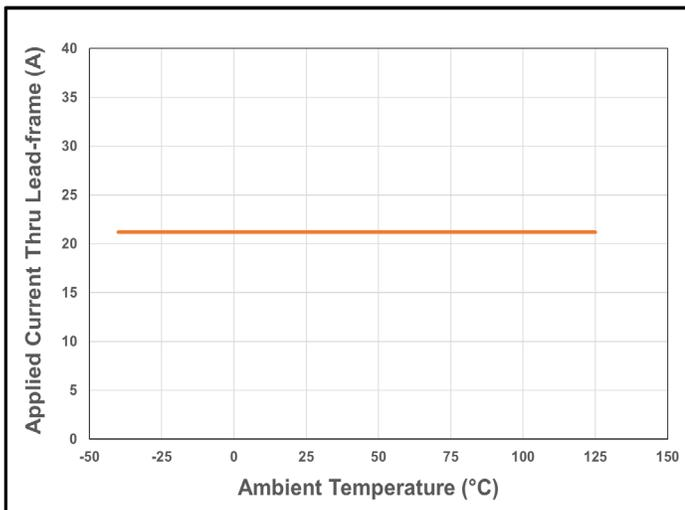
Figure 22. CT426 Current De-rating Curve for 30 A<sub>PK</sub> (21.2 A<sub>DC</sub>)
