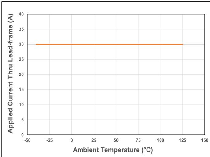
**Figure 19. CT426 Current De-rating Curve for 30 A<sub>DC</sub>**
