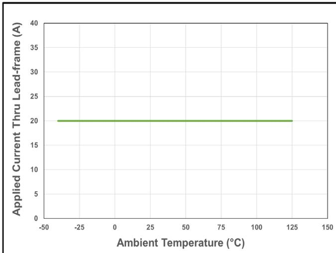
Figure 13. CT426 Current De-rating Curve for 20 A<sub>DC</sub>
