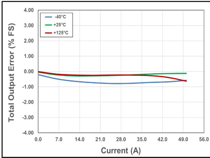
Figure 23. Total Output Error vs. Current vs. Temperature
