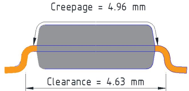
**Figure 39. The Creepage and Clearance for the CT426's SOIC-8 package**
