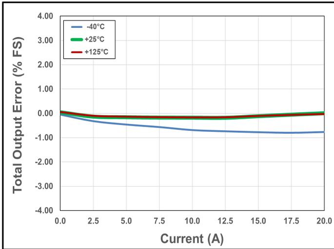
Figure 11. Total Output Error vs. Current vs. Temperature
