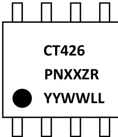
Figure 45. CT426 Device Marking for 8-lead Package
