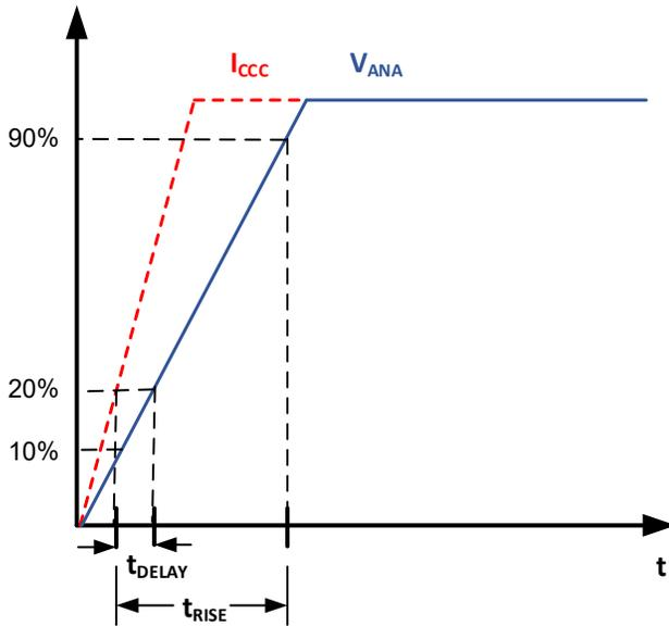
**Figure 38. CT426 Propagation Delay and Rise Time Curve**
