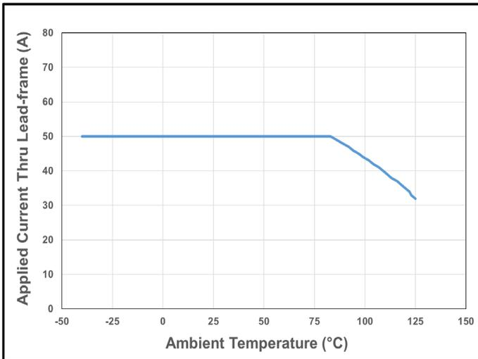
Figure 25. CT426 Current De-rating Curve for 50 A<sub>DC</sub>
