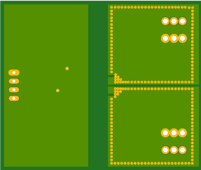
Figure 42. Recommended PCB Layout (Bottom Layer) for the 20 A to 65 A variants of the CT426.
