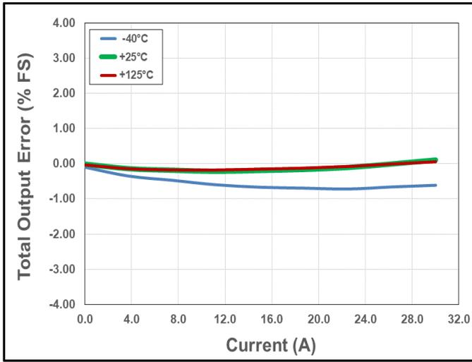
**Figure 17. Total Output Error vs. Current vs. Temperature**
