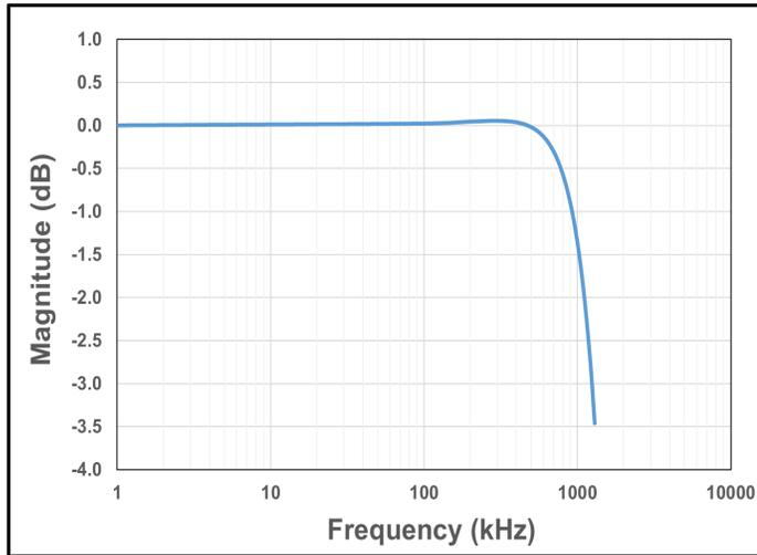
Figure 7. CT426 Bandwidth with  $C_{FILTER} = 1.0\ \text{pF}$
