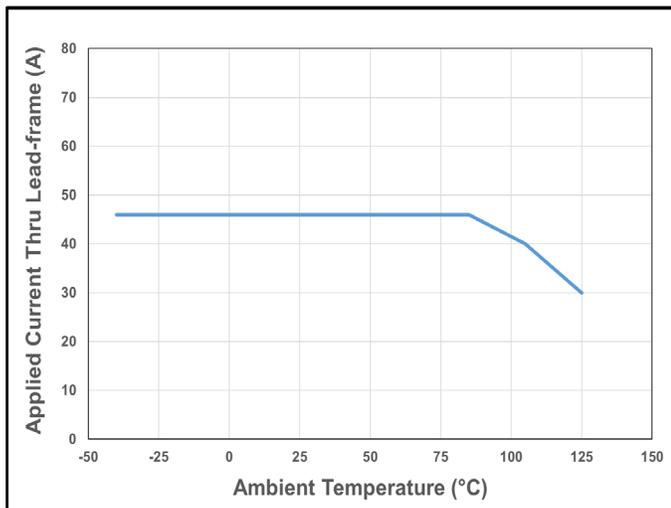
Figure 34. CT426 Current De-rating Curve for 65 A<sub>PK</sub> (46.0 A<sub>DC</sub>)
