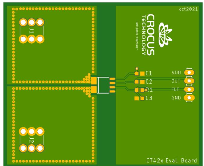
Figure 41. Recommended PCB Layout for the 20 A to 65 A variants of the CT426.
