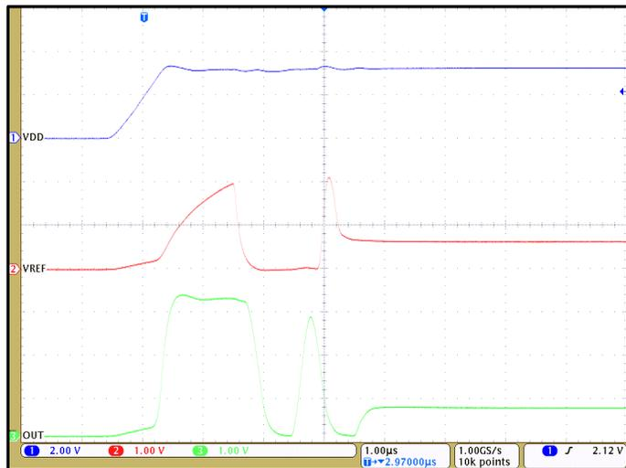
Figure 5. CT426 Startup Waveforms for  $V_{OQ} = 0.65\text{ V}$
