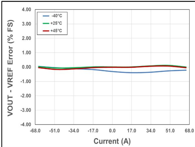
Figure 32. Total Output Error vs. Current vs. Temperature
