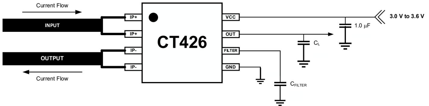
Figure 40. CT426 Application Block Diagram
