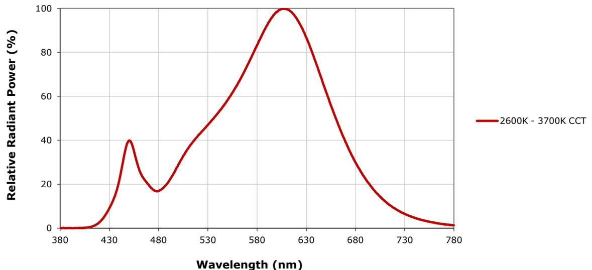
**RELATIVE SPECTRAL POWER DISTRIBUTION (48 V, 22 mA; T<sub>j</sub> = 85 °C)**
