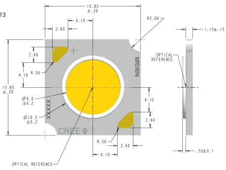
Tc measurement point: either the anode or cathode solder pad
