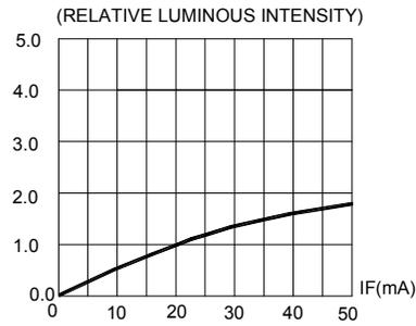
FIG. 2 RELATIVE LUMINOUS INTENSITY VS. FORWARD CURRENT
