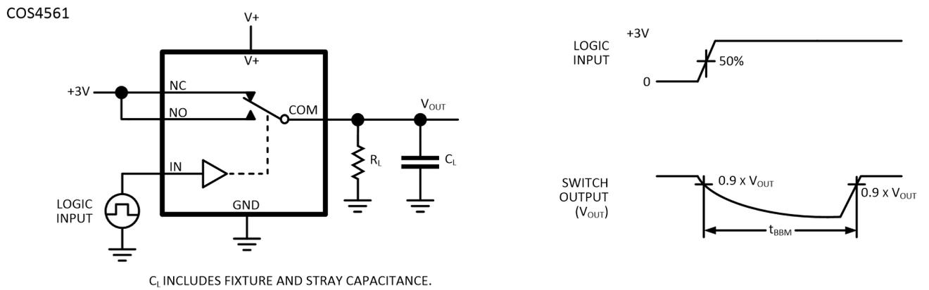
Figure 2. Break-Before-Make Interval
