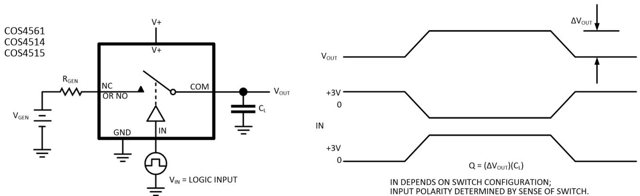
Figure 3. Charge Injection
