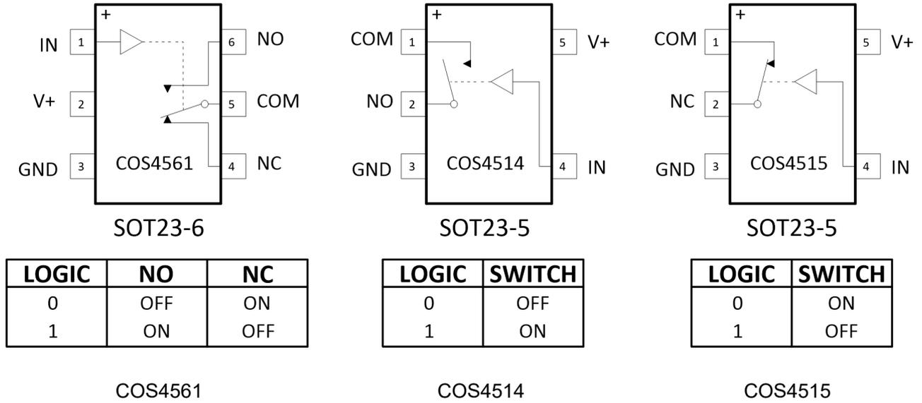
Figure 1 Pin Diagram
