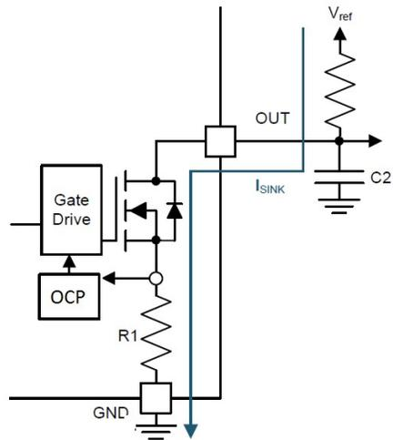
Select a value for C2 based on the system bandwidth specifications as shown in [Equation 2](#).
