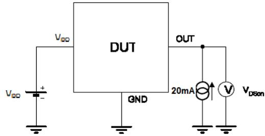
Note 1 - The output saturation voltage  $V_{DSon}$  is measured at  $V_{DD}=3.8V$  and  $V_{DD}=24V$
