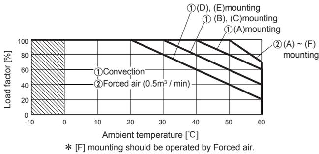
● LGA150A-□-SN (with Chassis & Cover) Ambient temperature derating curve
