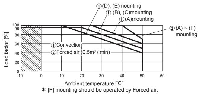
● LGA240A-□ Ambient temperature derating curve
