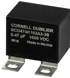
Style SCD offers protection against voltage transients in low to medium current IGBT applications where high dV/dt is encountered. Connect these capacitors from C1 to E2 on a dual IGBT module or from P to N on a six-pack module to eliminate severe voltage transients. Parts ending with Z25 fit IGBTs with 23mm, 25mm and 28mm lead spacing. If you have a preferred lead spacing, please specify.
