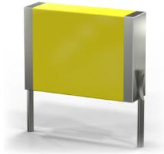
The RA style capacitor is constructed in an efficient rugged self-encased size. The non-inductive multilayer metallized polyester film capacitor features a small size, high dv/dt capability, very low ESR at high frequency and a self-healing capability. RA type capacitors are ideal for use in high frequency switching power supplies, noise suppression, EMI reduction and long-life applications.
