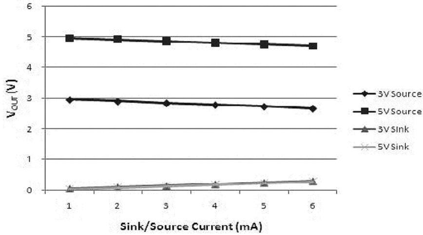
Figure 9. Vout Source and Sink Current Capability
