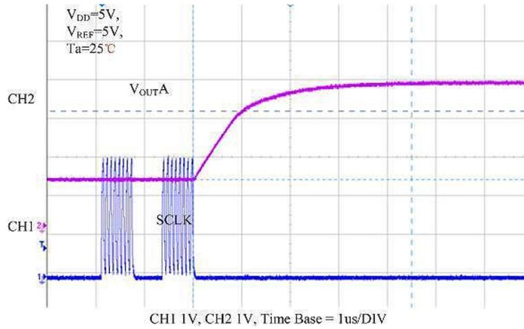
Figure 10. Half-scale setting (0.25 to 0.75 Scale Code Change)
