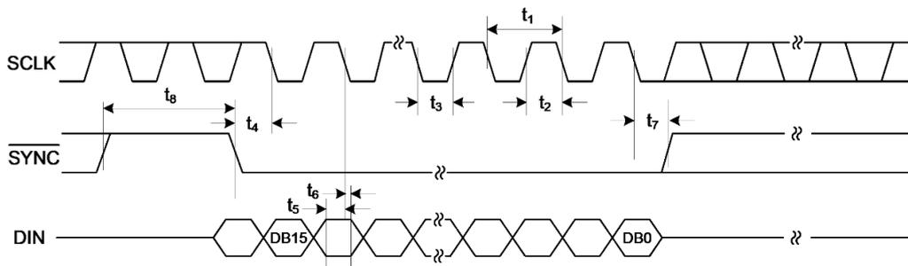
Figure 3. Serial Interface Timing Diagram
