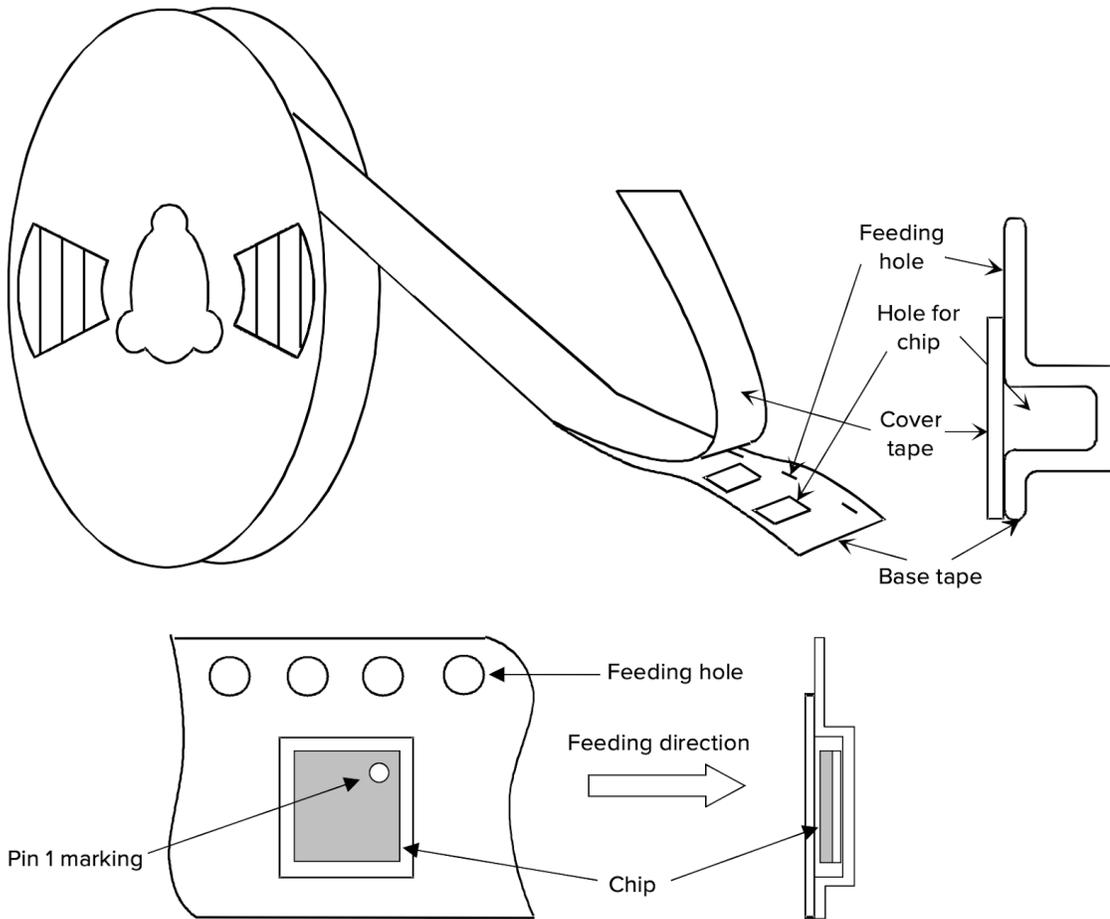
**Figure 13.** Taping diagram
