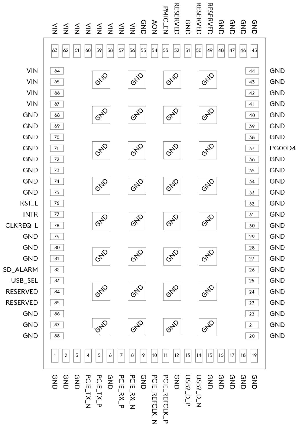
Figure 2. Pin names and numbers (top view)
