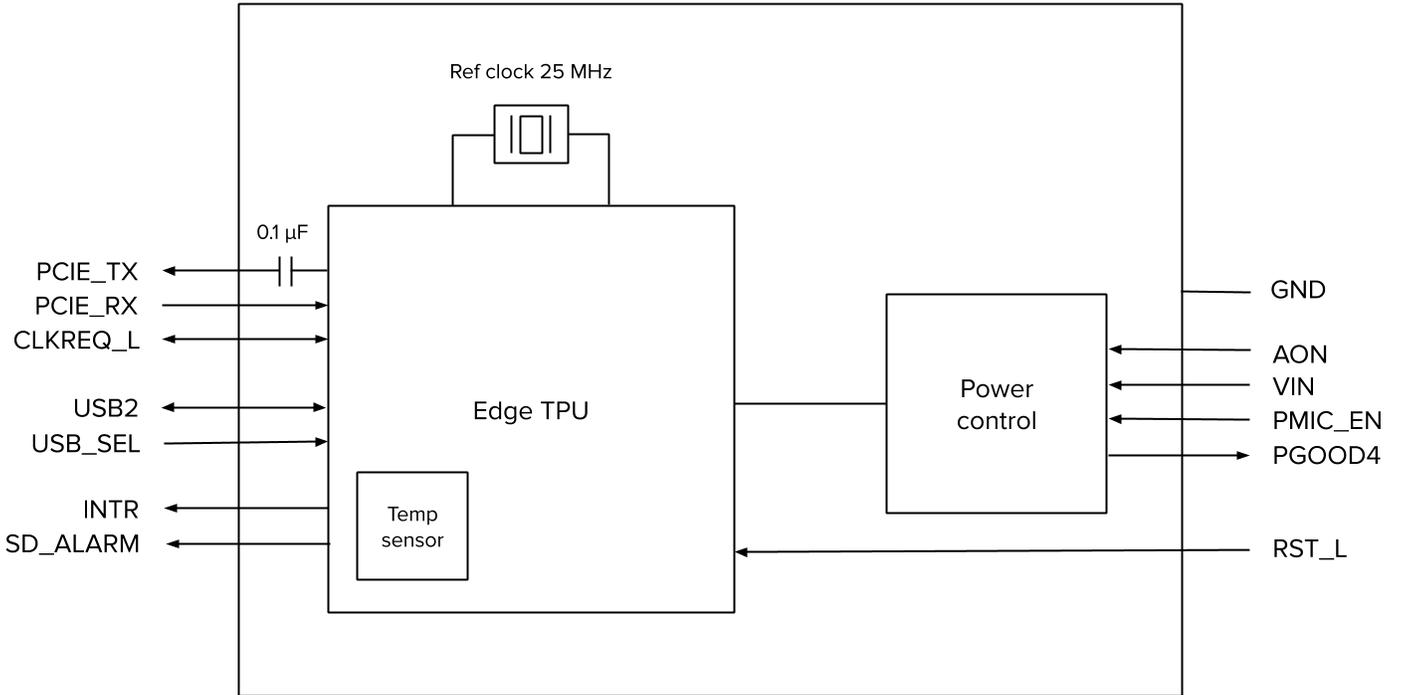
**Figure 1.** Accelerator Module functional block diagram
