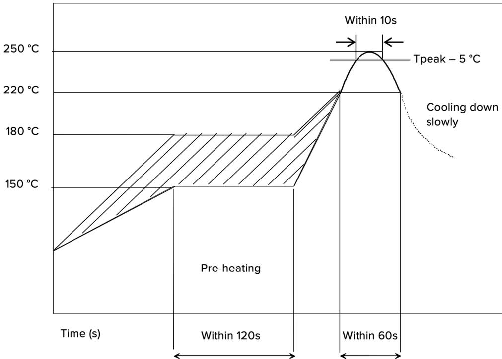
Figure 10. Reflow soldering conditions example
