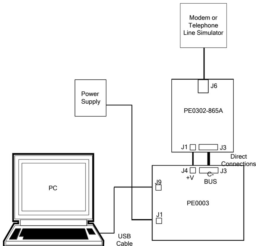
Figure 2 PE0302-865A used with PE0003
