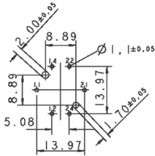
PCB hole pattern, component side
