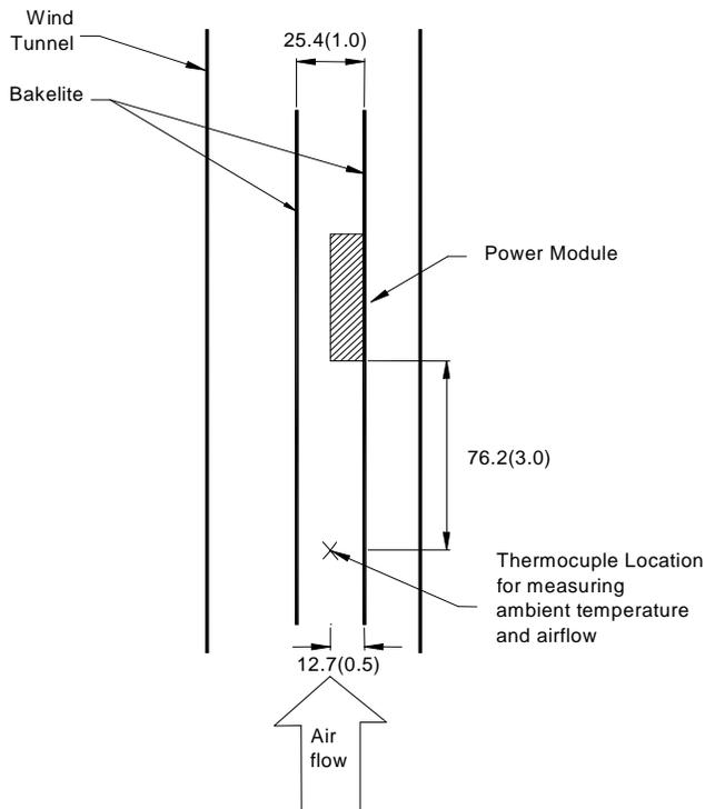
Note : Dimensions are in millimeters and (inches)
