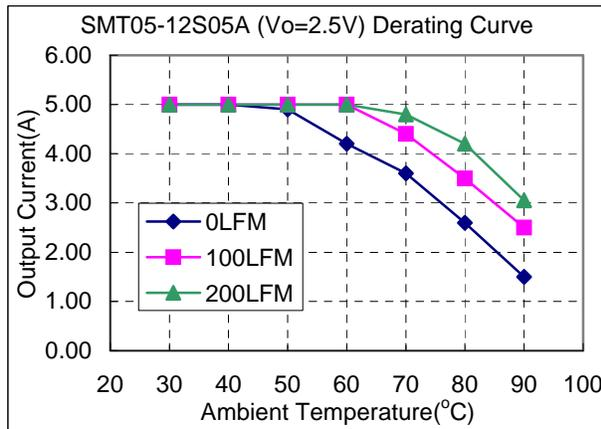
Figure12c. Typical Power De-rating for 12V IN 2.5Vout
