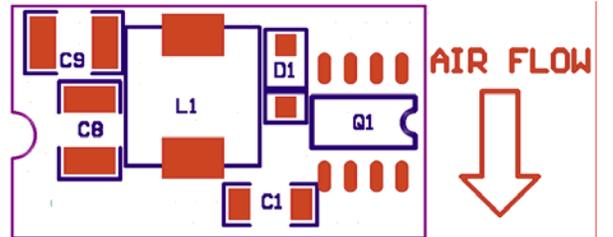
Figure 9. Temperature Measurement Location for SMT
