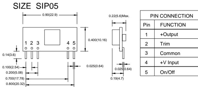
Figure 20 SIP05 Mechanical Outline Diagram
