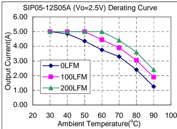
Figure 10c. Typical Power De-rating for 12V IN 2.5Vout
