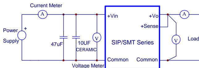
Figure 15. SIP/SMT05-12S05A Test Setup
