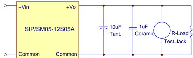
Figure 18. Output Voltage Ripple and Noise Measurement Set-Up
