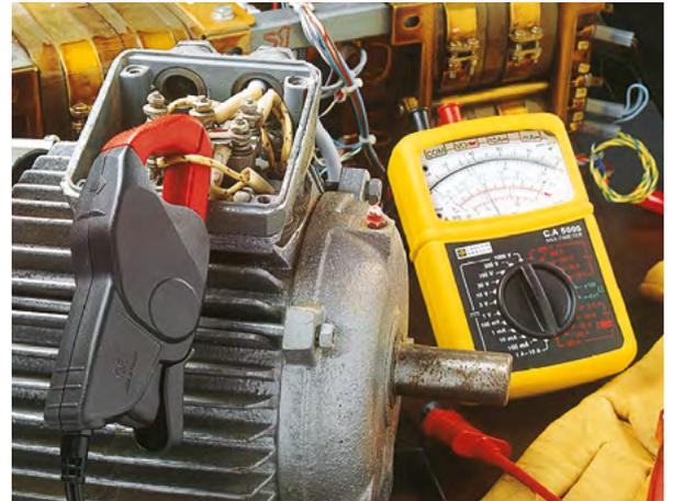
▲ **Direct reading of the motor current with the C.A 5005 and its MN 89 miniclamp,** supplied as standard. The A AC ranges are marked by the
