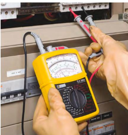
**Continuity test™ of a fuse with the C.A 5001.** The jointed clip is folded in place as a stand for use on the workbench. ▶
