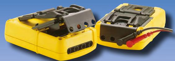
It is essential to disconnect the leads before opening the cover for access to the battery and the fuses. Rapid opening by 1/4 turn screw, using a coin or a screwdriver.
