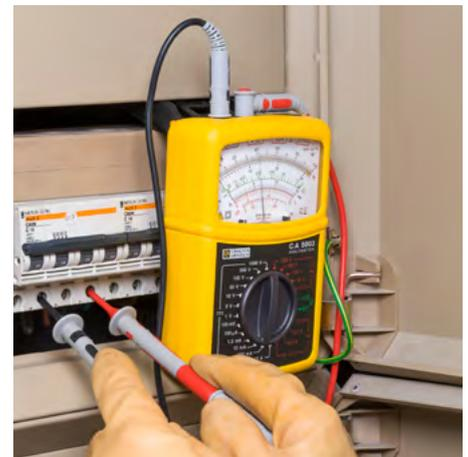
▲ **The articulated stand** holds the C.A 5003 in a vertical position for a reading close to the test point.
