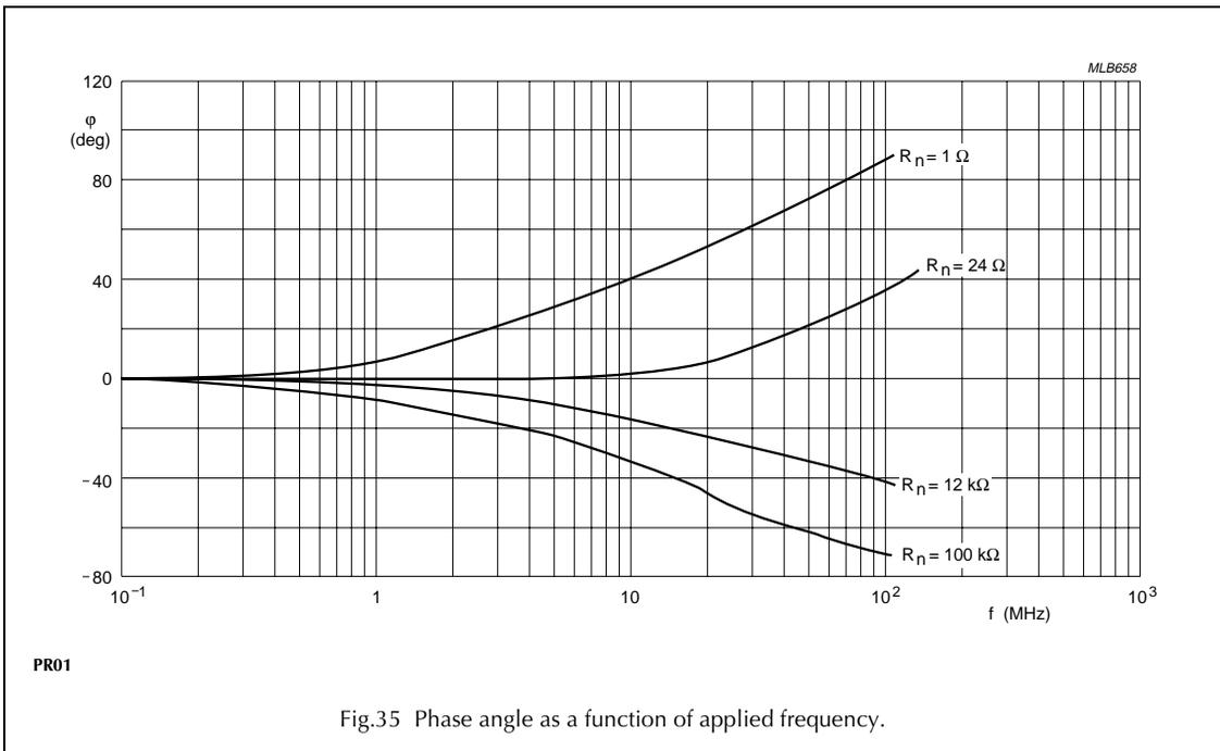
Fig.35 Phase angle as a function of applied frequency.
