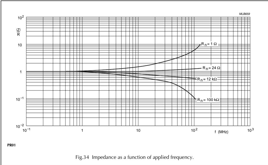
Fig.34 Impedance as a function of applied frequency.
