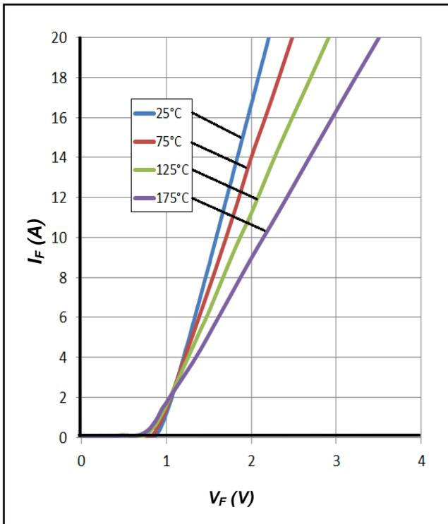
Figure 1. Forward Characteristics
