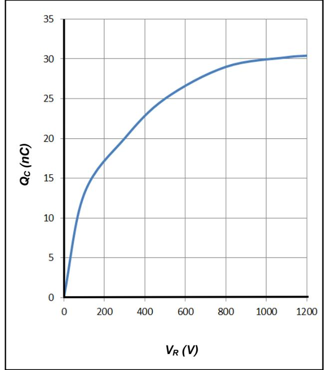
Figure 4. Total Capacitive Charge vs. Reverse Voltage
