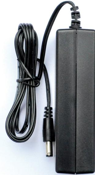
The **CL12.6VDC-4.76A** is a high-performance and efficient 4.7 A charger for lithium-ion batteries in a small desktop enclosure. It supports 3S packets (three cells connected in series) and is designed to be charged at normal speed and to keep the batteries ready. Its design is based on high-quality electronic components that allow for continuous, long-term operation in all conditions.
