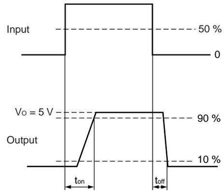
★ TYPICAL CHARACTERISTICS ( $T_A = 25\text{ }^\circ\text{C}$ , unless otherwise specified)
