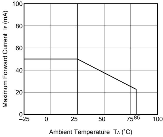
MAXIMUM LOAD CURRENT vs. AMBIENT TEMPERATURE
