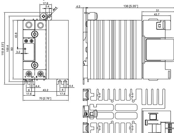
Housing width tolerance +0.5mm, -0mm as per DIN 43880. All other tolerances +/- 0.5mm. Dimensions in mm.
