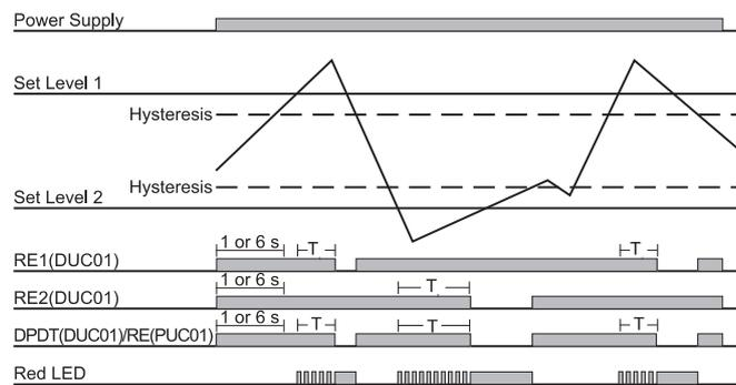
**Over+under voltage - Latch - N.D. relay(s)**
