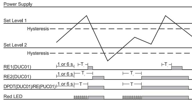
**Over+over voltage - Latch - N.D. relay(s)**
