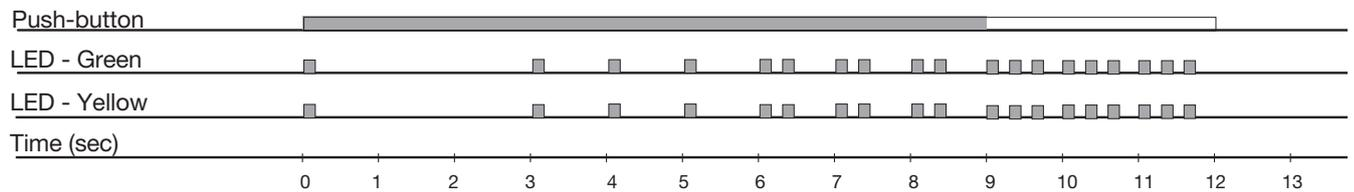
Releasing the push-button after 12 sec. will reset the sensor to factory settings.
