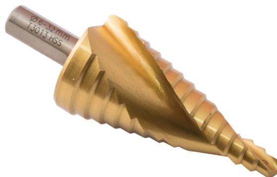
**Features & Benefits** ~ Centres, drills and deburs sheet metals in one operation ~ Titanium coated for longer life ~ HSS, precision ground for accurate drilling ~ Dual flute construction for faster drilling & longer life ~ Three flats on drive shaft for secure drive in drill chucks ~ Cuts hole sizes: 6, 8, 10, 12, 14, 16, 18, 20, 22, 24, 26, 28, 30 & 32 mm
