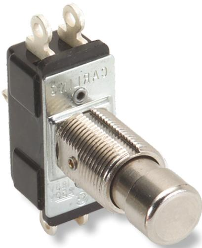
The 110/316P-Series provides a compact yet rugged solution to general purpose switch needs. Alternate action, metal construction and stiff (6-8 lb) actuation force have combined to make this switch a pillar in a variety of markets. This versatile switch is available in maintained and momentary circuits with a variety of termination and rating options.
