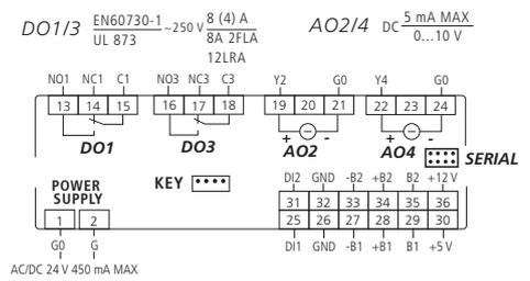
2.5 IR33/DN33 Universale with universal inputs - probe connections
