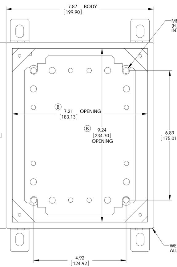
M8 x 16mm LG. WELD STUD/STANDOFF (4x) (FLAT WASHER, LOCKWASHER & HEX NUT FOR INTERNAL PANEL MOUNTING)
