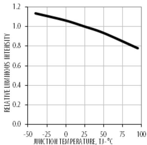
**Figure 7 Derating Curve**
