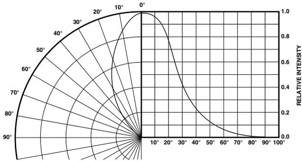
Figure 4. Relative luminous intensity vs. angular displacement for T-1<sup>3/4</sup> lamp.
