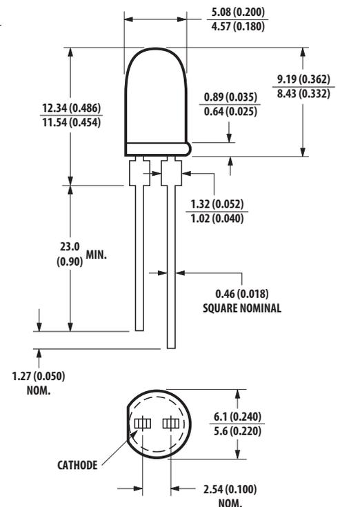
**Figure B. T-1<sup>3</sup>/<sub>4</sub> package.**
