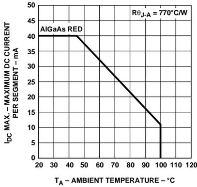
Figure 2. Maximum Allowable DC Current vs. Ambient Temperature.
