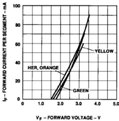
Figure 10. Forward Current vs. Forward Voltage Characteristics.
