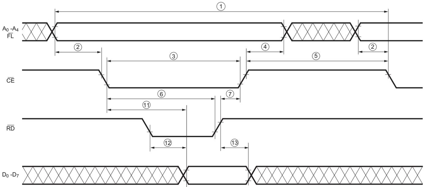
INPUT PULSE LEVELS: 0.6V to 2.4V
