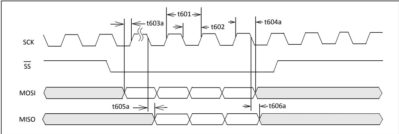
**Figure 36: SPI Timings,  $\overline{SS}$  Asserted During SCK Low**
