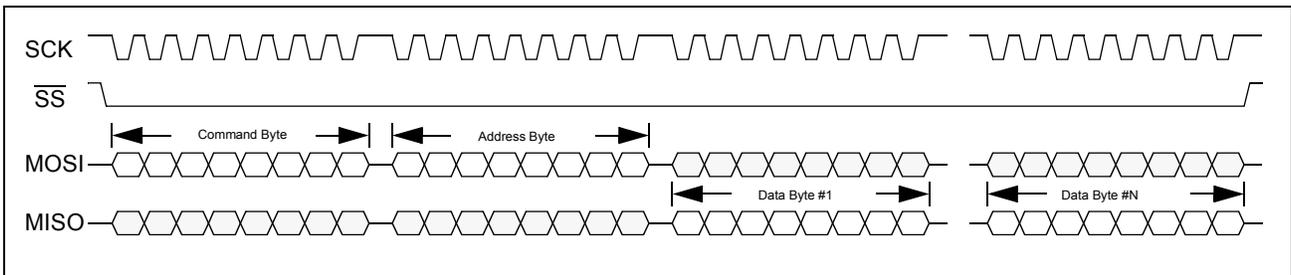
The Serial interface supports operation up to 2 MHz in SPI mode. A maximum of four devices can be cascaded/ addressed.
