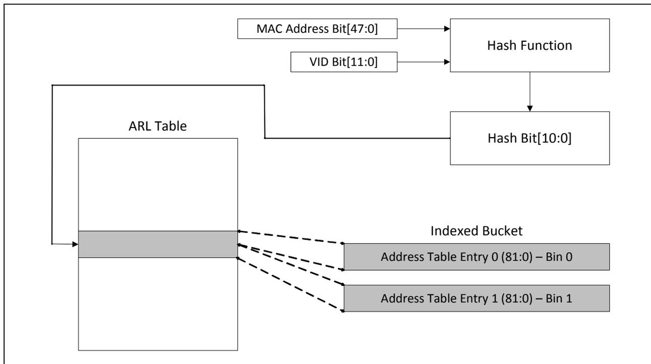
The index to the address table is computed using a hash algorithm based on the MAC address.
