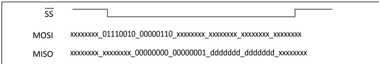
Write operations are identical in fast and normal SPI mode.
