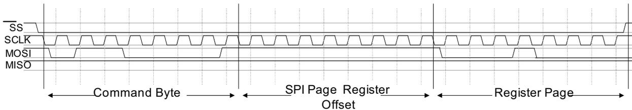
3. Issue a Fast Read command (opcode = 0x10), followed by the Address of the accessed register (0x12), check for a read completion by checking the RACK bit in the SPI Status register, and finally clock out the read data.
