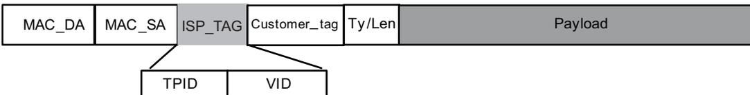
The switch uses the ISP tag for ARL and VLAN table accesses and the customer tag as an IEEE 802.1Q tag. There is a per-chip programmable register Double Tagging TPID register for ISP tag (default = 9100'h). All ISP tags will be qualified by this Tag Protocol ID (TPID) value.
