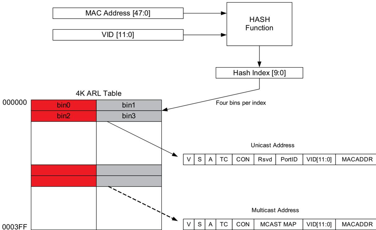
The index to the address table is computed using a hash algorithm based on the MAC address and the VLAN ID (VID) if enabled.
