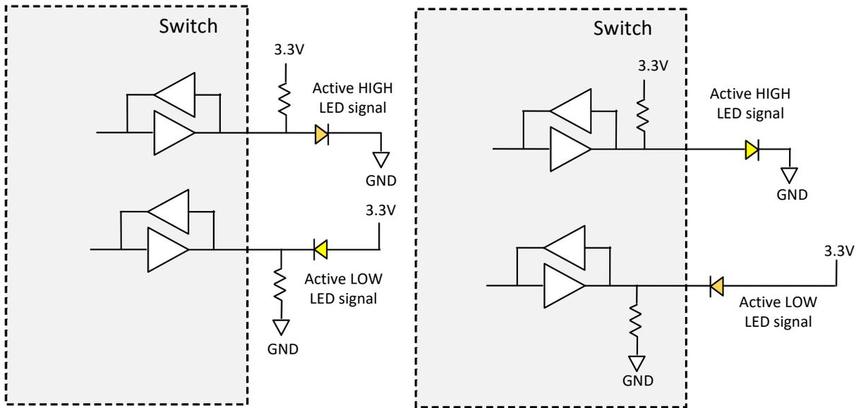
**Note:** When LED signal pins are pulled up or down through an external or an internal termination due to the strap pin configuration, the active states of LED signals are as follows:
