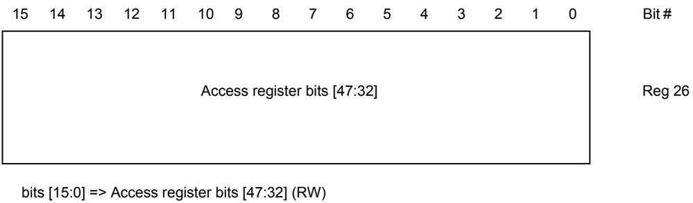
**Figure 41: Pseudo-PHY MII Register 27: Access Register Bit Definition**
