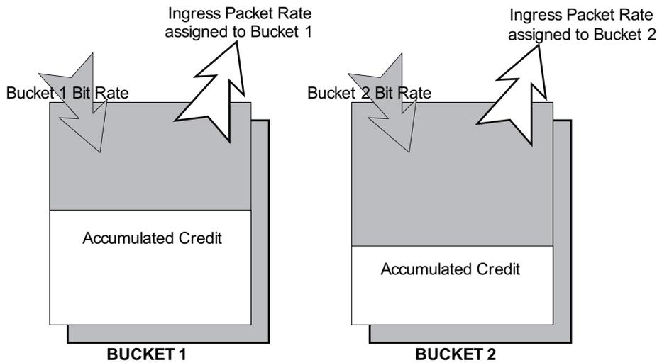
If there is no accumulated credit available, the switch does not accept input packets.
