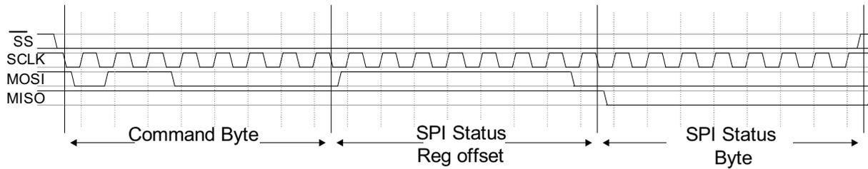
2. Issue a Normal Write command (opcode = 0x61) and write the accessed register page value of 0x10 in to SPI Page Register(0xFF)—this step is required only if previous read/write was not to/from Page 10h.
