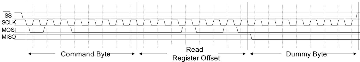
**NOTE:** This dummy read is always eight clock cycles, whether or not it is an 8-bit register.
