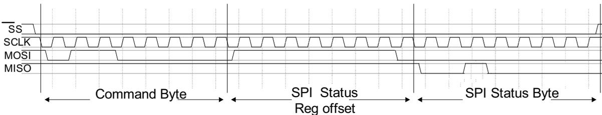
5. Issue a Normal Read command (opcode = 0x60) to read the data from the SPI Data I/O register:
