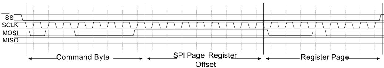
3. Issue a Normal Read command (opcode = 0x60) and write the accessed register address value 0x12, and clock out 8 bits to complete the read cycle, but discard result (this is where the state machine triggers an internal data transfer from address 0x12 to the SPI Data I/O register).
