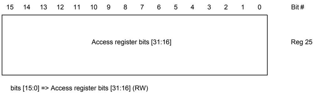
**Figure 40: Pseudo-PHY MII Register 26: Access Register Bit Definition**
