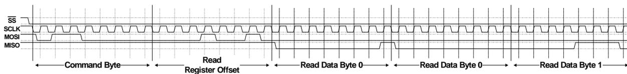
**NOTE:** There is an erratum on the RACK output timing in Fast Read mode. The RACK (bit 0) must be sampled prior to toggling the clock to shift out the bit 0.
