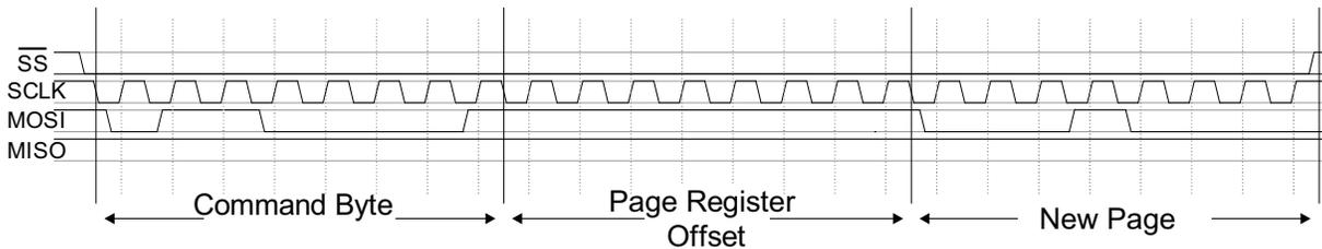
3. Issue a Normal Write command (opcode = 0x61) and write the Address of the accessed register followed by the write content starting from a lower byte.
