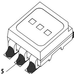
$T_S$  can be measured easily by mounting a thermocouple on the soldering joint as shown in preceding illustration, while  $R_{\theta J-S}$  is provided in the data sheet. Verify the  $T_S$  of the LED in the final product to ensure that the LEDs are operated within all maximum ratings stated in the data sheet.
