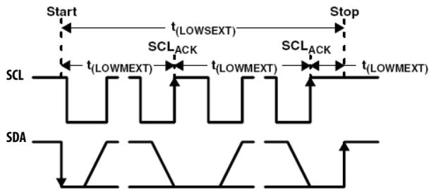
**Figure 1. I<sup>2</sup>C Bus Timing Diagram**
