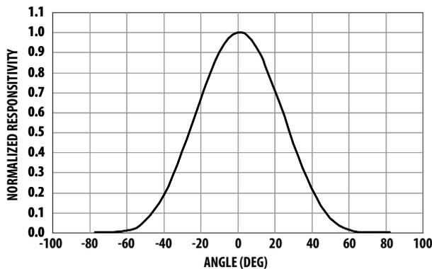
Figure 5. Normalized ALS Response vs. Angular Displacement
