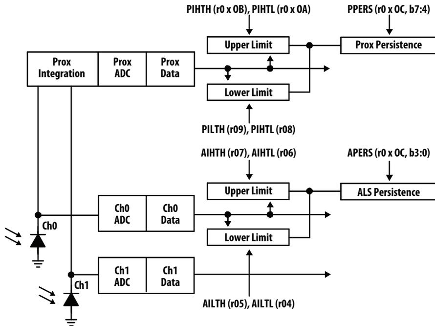
Figure 12. Programmable Interrupt
