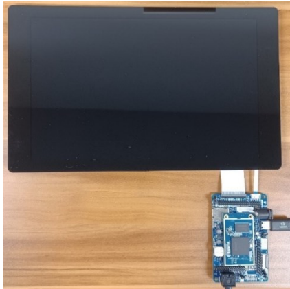
Figure 16 - VM820C Setup with 10.1" 1920 x 1200 LCD Panel
